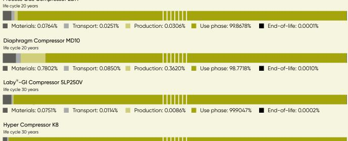
The vast majority of emissions over the entire life cycle of a compressors are caused in the use phase due to the high power range of our compressors, their long lifetime and their uninterrupted operation.
